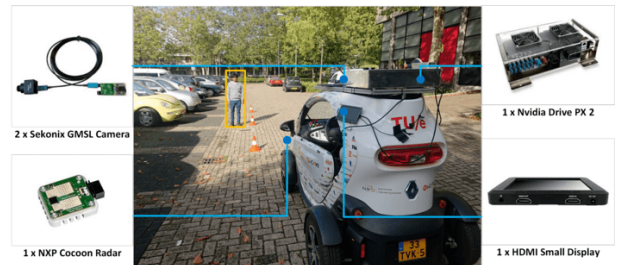
Fig. 9: The experimental setup of the Twizy cooperative automated research vehicle platform.
