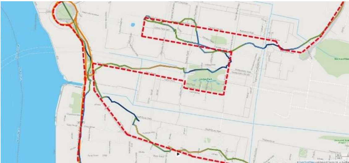
Figure 2-2: Output from a Garmin Forerunner 935 GPS device compared to a known route through London’s Canary Wharf, an area with numerous skyscraper buildings. Colour toned line represents GPS estimated location. Red dashed line represents true route followed.
