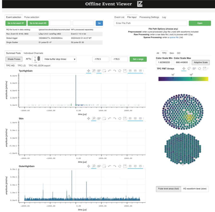
Figure 4.1: A CH 3 T calibration event in the TPC visualised using the LZ Offline Event Viewer. The PMT hitmap in the TPC is shown on the right along with the summed waveform in the TPC, Skin Detector and OD shown in the three panels on the left.
