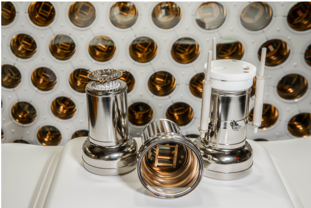
Figure 3.4: A photograph of the Hamamatsu R11410-22 3" PMTs used in the LZ TPC taken by Matthew Kapust, Sanford Underground Research.
