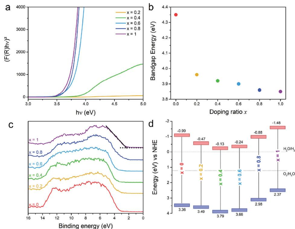
**Figure 5.** Optical and electronic properties of the Ti/Ge samples as a function of the substitution ratio: a) Tauc plots; b) evolution of the band gap energy  $E_g$ ; c) XPS spectra in the VB region and d) corresponding energy diagram scheme.
