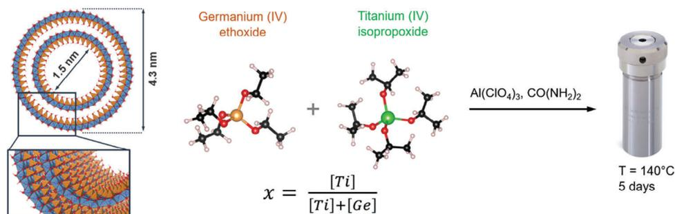
**Figure 1.** (Left) Schematic view of a DWINT structure with Al, Ge, and O atoms represented in blue, orange, and red, respectively. (Right) The proposed method to dope imogolite nanotubes with Ti atoms at different precursor ratio  $x$ .
