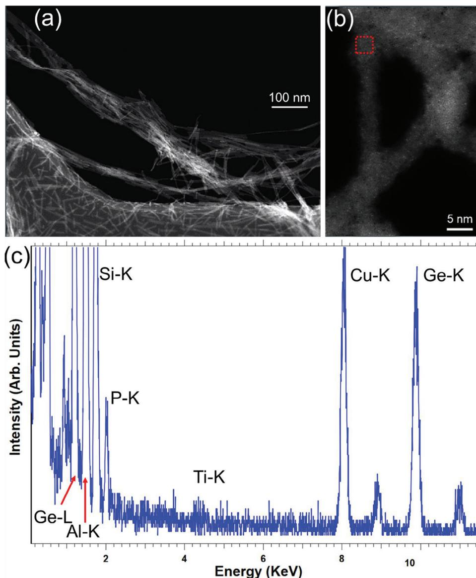
**Figure 4.** Scanning transmission electron microscopy (STEM) analyses of imogolite nanotubes. a,b) High-angle annular dark field (HAADF)-STEM micrographs. c) XEDS spectrum acquired from the red highlighted area in panel (b) on an individual nanotube. Titanium has been detected in this region of the nanotube as visible from the signal in the Ti-K X-ray emission.
