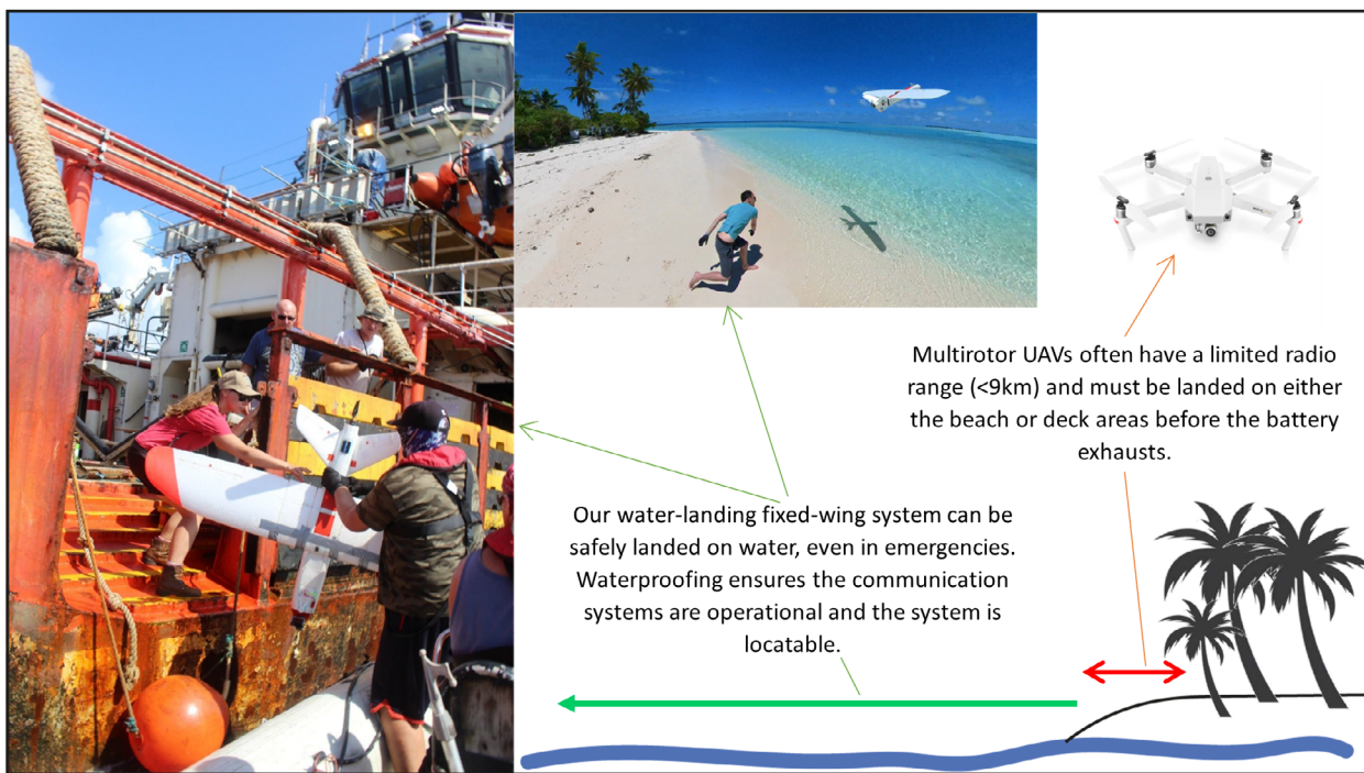
Figure 1. The UAV system is handed back to the pilot by the daughter craft crew, after retrieval from a successful water landing, in 2018. We outline how limited landing opportunities are for multirotor UAVs on many small islands, and in emergencies, this can jeopardise system safety if there is an accidental water landing. Photograph courtesy of Three Wise Monkeys production company and Oceans Unmanned.
