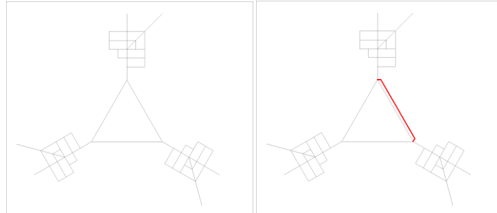
Figure A. Two notional network models: street-only (A) and multi-modal (B) with a fast link (red)
