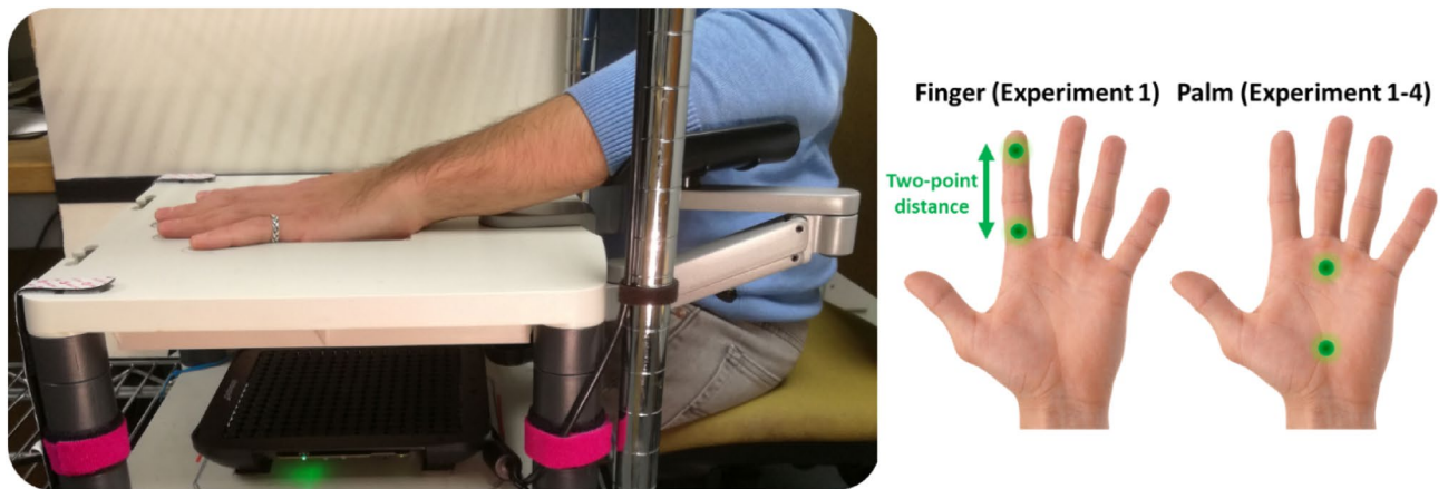
Figure 1. Experimental setup for Experiments 1–3. The participants sat at a desk, resting their left elbow on an articulated armrest support and their left hand palm down on a plastic support, in correspondence of a 10 \times 10 cm aperture. The view of the left hand was blocked by a fixed vertical plywood screen throughout the entire experiment. Airborne ultrasound stimulation was delivered through a STRATOS Explore device located 12 cm below the participant's hand. In Experiment 1, tactile stimuli were delivered either on the index finger or the palm of the hand. Given that Experiment 1 did not find a significant effect of the location of stimulation in Experiments 2–4 stimuli were delivered to the palm only.
