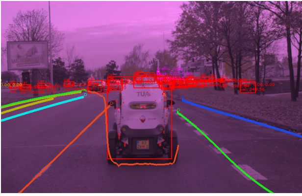
Fig. 11: Results of Stereo Vision System with Vehicle.
