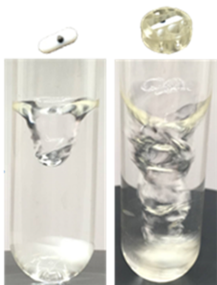
Figure 5. Vortexing ability of a conventional stirrer at 1400 rpm (left) versus that of its 3D-printed congener (right).
