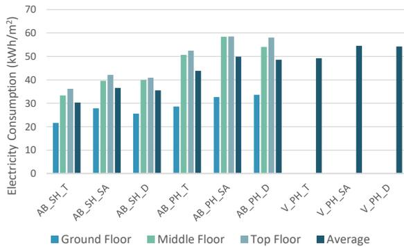
Figure 10 - Simulated electricity consumption intensity.
