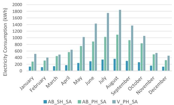
Figure 11: Simulated monthly electricity consumption for the semi-attached archetypes.
