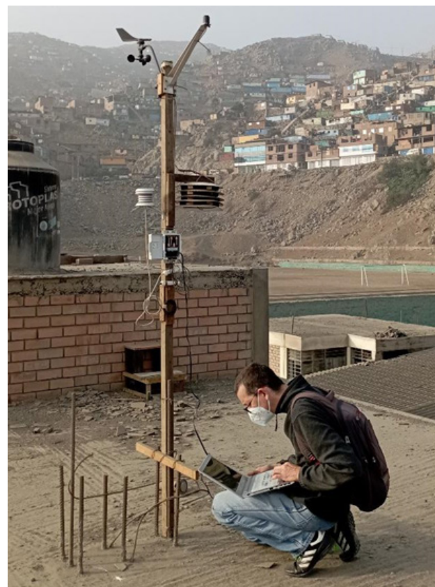
Figure 1: Checking the results from weather station installed in José Carlos Mariátegui. Photo: Marion Verdier
