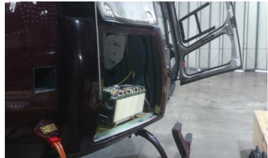
Figure 12 AEXAR installed in a Twin Squirrel Helicopter
