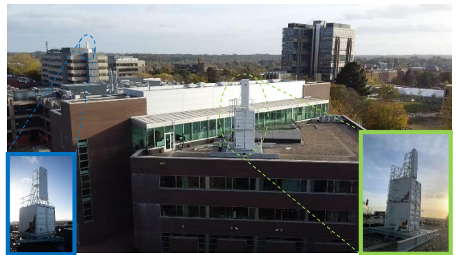
Figure 5 Two L-Band multiple receive beam staring radar installed at University of Birmingham Edgbaston campus.
