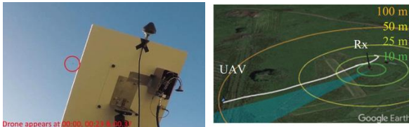
Figure 1 GNSS based passive radar setup (left) and example of acquisition scenario (right).
