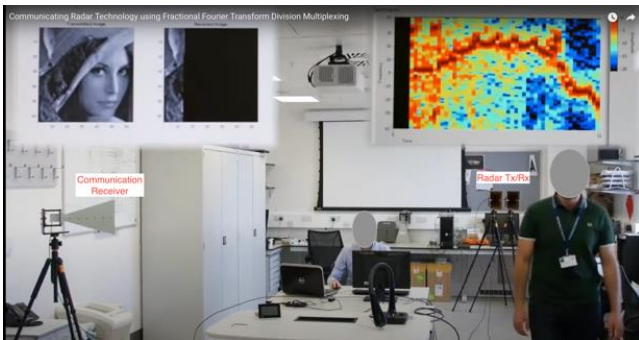
Figure 2 Software Defined Radio based joint radar and communication system
