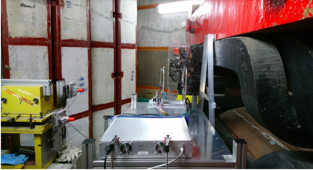
Figure 4.12.: A photograph of the initial electron region of the test-beam setup. The beam emerges from the left. The two detector planes are visible in the centre, and the thin tungsten target is flush to the edge of the magnet in a metallic frame.
