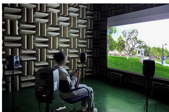
Fig. 4. Setup of audiovisual reproduction system.
