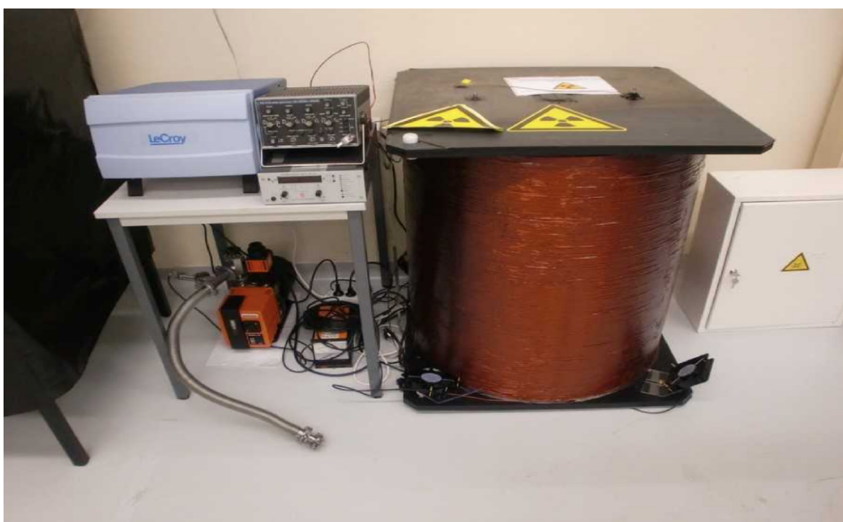
Figure 3.17: Image of the copper solenoid and impermeable container used to measure the ability of the shields to remove the magnetic field within their volume [123].
