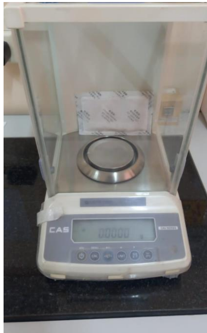
Fig. 5.22 Analytical grade scales used to determine the weight of rebars after the pickling with Clark's solution.
