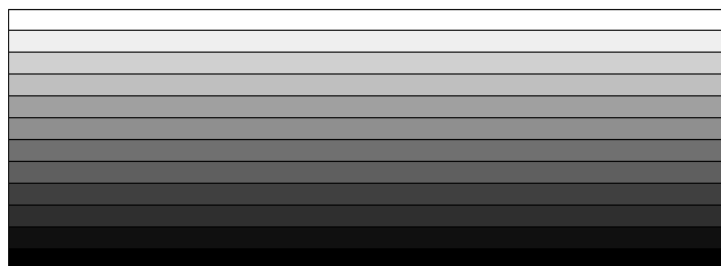
Figure 3. Uniform division of an FG-porous CNTRC beam into homogenized sub-layers.
