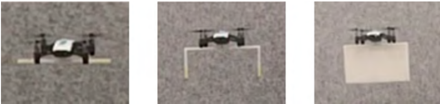
Figure 7. Demonstration: carrying different objects to perform different tasks (e.g., frame, layer, and holders).
