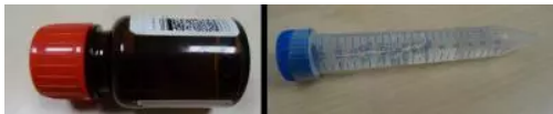
Figure 2: Phantoms used in the study. Left: Simple bottle phantom (diameter of 4 cm) filled with pure trifluoroethanol ( \text{C}_2\text{H}_3\text{F}_3\text{O} ) for testing the coil design; right: 15 ml falcon tubes with different concentrations of trifluoroethanol dissolved in \text{H}_2\text{O} (distilled water).
