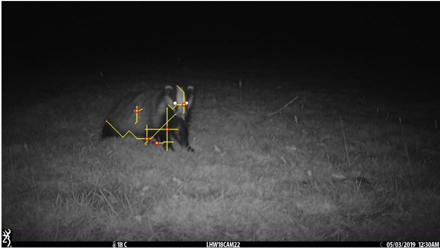
FIGURE 5 An illustration of five realisations of the 'bouncing' procedure. The starting points are shown by red circles, and the bouncing paths are shown by yellow lines. Note that the lines are of width four pixels to improve their visibility, although each considers only a single pixel at a time.
