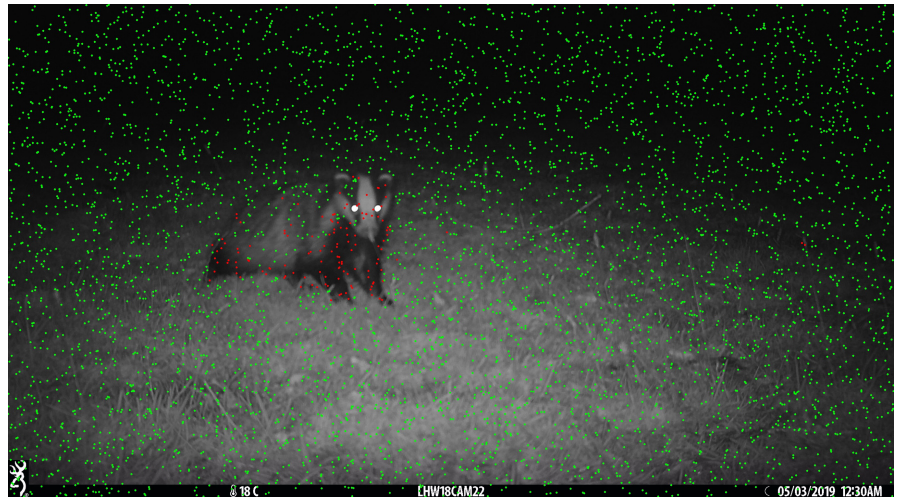
FIGURE 4 A graphic showing the result of sampling 5000 random pixels image I in Figure 2. Green circles indicate that a pixel was not counted as a disturbance, while red pixels indicate that a pixel was counted as a disturbance. Note that the circles have been set to have a radius of 3 pixels for demonstrative purposes although only a single pixel was analysed in each case.
