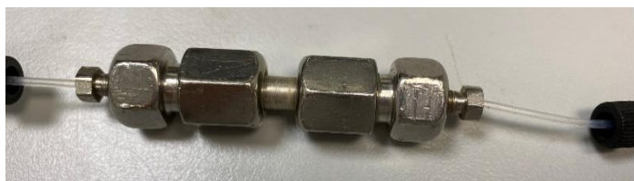
Figure 2.7: Diels-Alder packed-bed reaction with aluminium chloride immobilised on silica gel.
