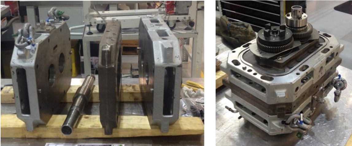
Figure 37 Left showing dismantled pump, right showing pump back together with gears on top and throwers sitting below, outer casing yet to be attached on the side it is standing up on
