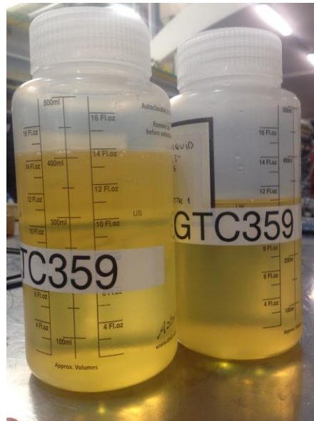
Figure 36 Scaled up sample of MIL9 ready to be added to the test pump, two containers combining multiple smaller scale preparations
