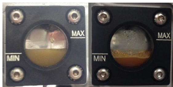
Figure 46 Oil display showing discolouration of lubricant on both gauges of the test pump
