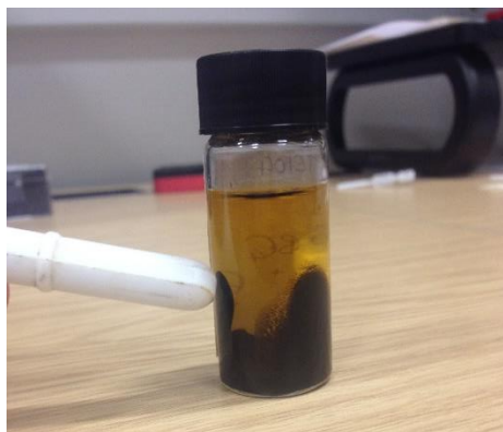
Figure 70 Nanoparticles synthesised in-situ showing a clear paramagnetic response to the white magnet seen in the figure
