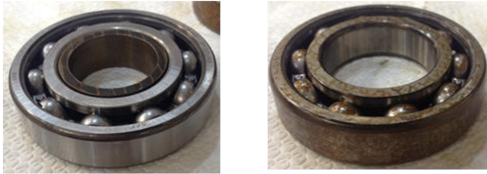
Figure 39 Early issue of corroded bearing (right) after being pre-lubed and left overnight
