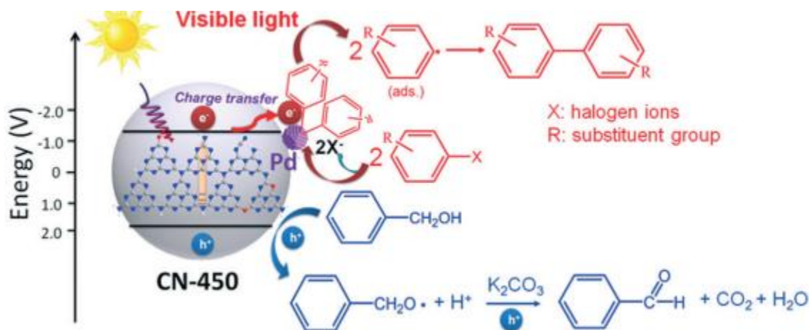
Scheme 28 Proposed mechanism of photocatalytic Ullmann coupling and aromatic alcohol oxidation over Pd/CN-450 [98]
