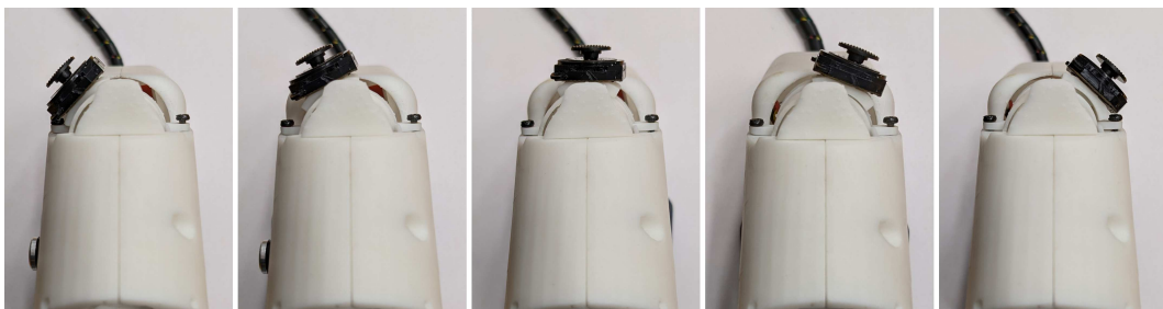
Figure 4.24: The rotating joystick-body in its 5 discrete positions with a rotating step of 15^\circ .
