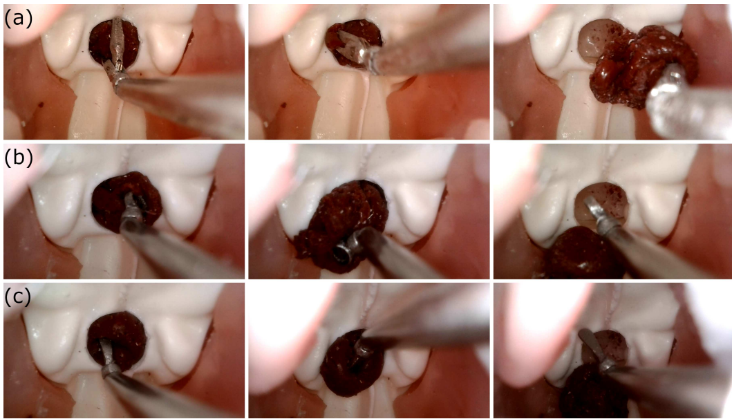
Figure 5.10: The view from the USB-endoscope during the phantom feasibility study where the silicone tumor at the pituitary gland region was removed with the use of (a). The robotic grasper, (b). The robotic ring-curette, and (c). The robotic dissector.
