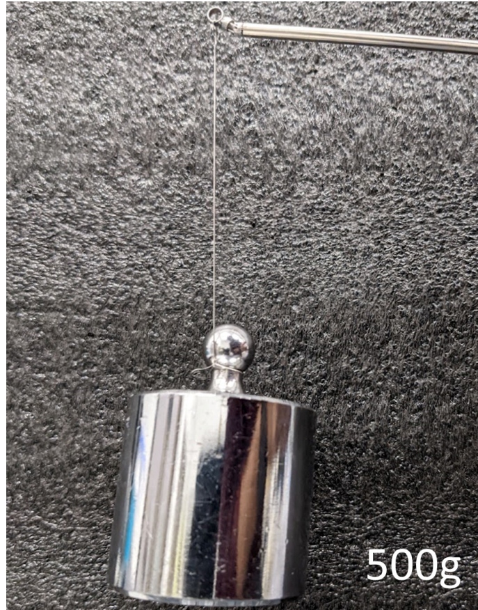
Figure 5.9: The ring-curette end-effector maintaining its pose holding a 500g weight.
