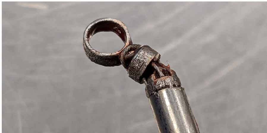
Figure 5.12: The miniature end-effector after the completion of the cadaver pilot study. In this figure, a snapped tendon strand can be seen.
