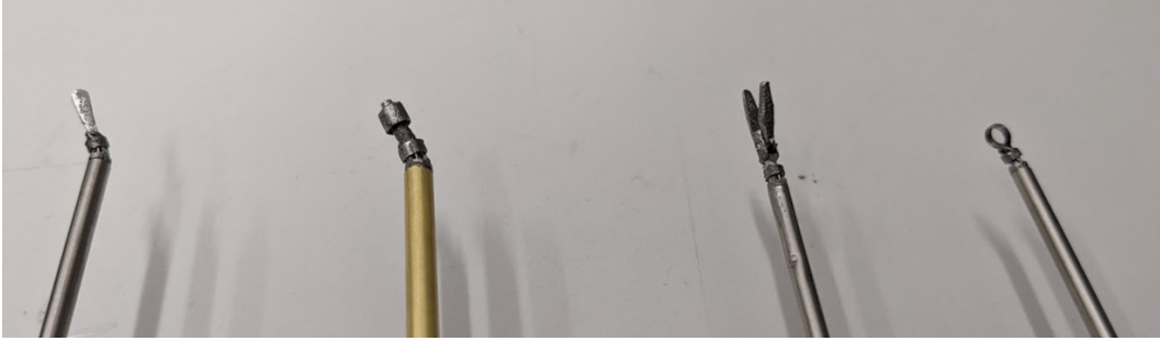
Figure 3.22: The articulated end-effectors developed as part of the novel robotic system. From left to right, a dissector, an endoscope, a grasper, and a ring-curette.
