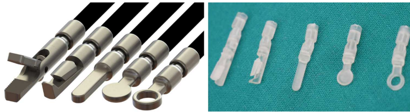
Figure 3.3: CAD renderings (left) and SLA-printed implementation of the end-effectors (right)
