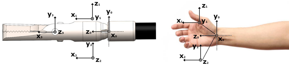
Figure 4.2: The coordinate frames of the end-effector that the handle is intended to manipulate (left), and the corresponding frames on the wrist (right).
