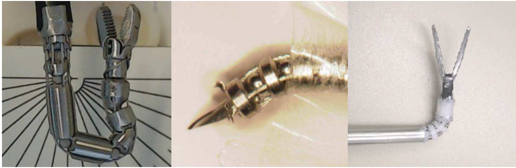
Figure 2.6: A surgical end-effector with a spherical joint that is part of a larger continuum body (left), an end-effector with two ball-joints that contribute towards an extended bending radius (middle), and an end-effector with an assembly of ball joints and plates (right).
