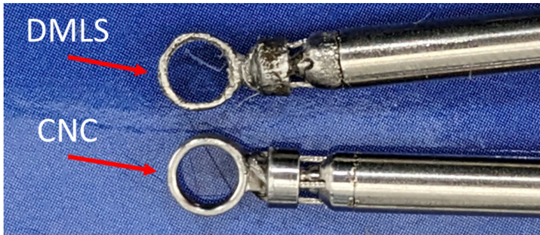
Figure 3.26: Comparison between an end-effector manufactured with DMLS and an end-effector manufactured with CNC machining.
