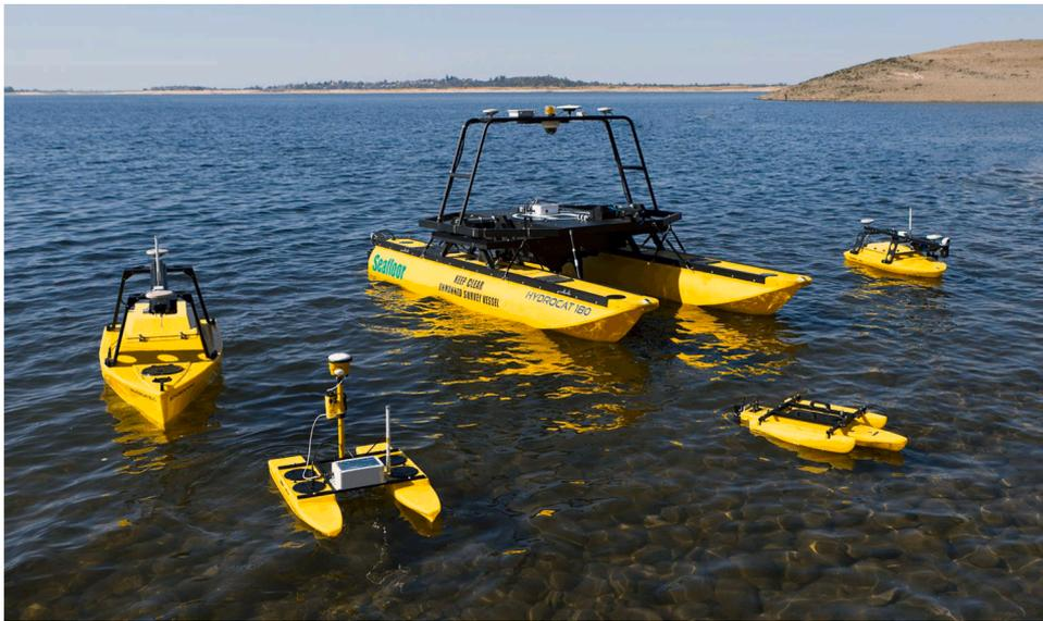
Fig. 1. Unmanned Surface Vehicle (USV) selection from Seafloor Systems, Inc. Image source: (Seafloor Systems).
