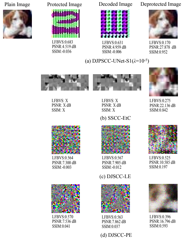
Fig. 10. Visually protected images comparison generated by DJPSCC-UNet-SC1( \lambda = 10^{-5} ), SSCC-EtC, DJSCC-LE and DJSCC-PE with the bandwidth ratio R=1/6 and \text{SNR}=10\text{ dB} . The image in the first column is the plain image. The images in the second column are the protected images transformed by the image owner. The images in the third column are the decoded images and the images in the last column are the deprotected images. (a) DJPSCC-UNet-SC1( \lambda = 10^{-5} ), (b) SSCC-EtC, (c) DJSCC-LE, (d) DJSCC-PE.
