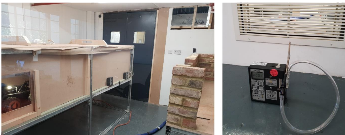
Figure 49. Setup of controlled room environment (left) and position of measurement for emissions near sprayer (right)
