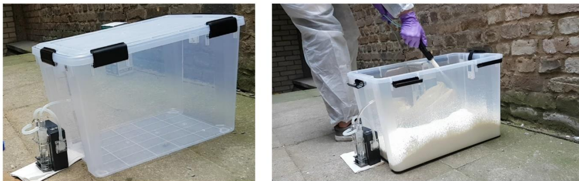
Figure 26. Experimental setup for isocyanate detection with the empty box (left) and the application of spray foam (right)
