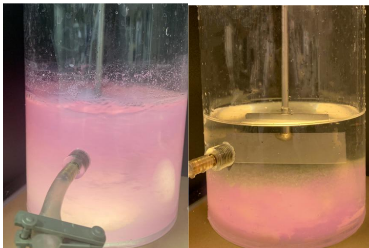
Figure 7. 2 Jar during the coagulation-flocculation process and after sedimentation (PS 5 mg/L PAC 0.4 mmol/L, PAM 3 mg/L, and 800 mL Regent's Park Pond water and Thames River water were used respectively. MPs that are coagulated-flocculated and settled are in pink colour.
