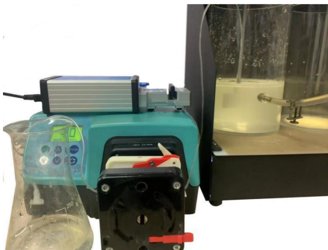
Figure 3. 1 PDA device and jar tester flocculator assembly
