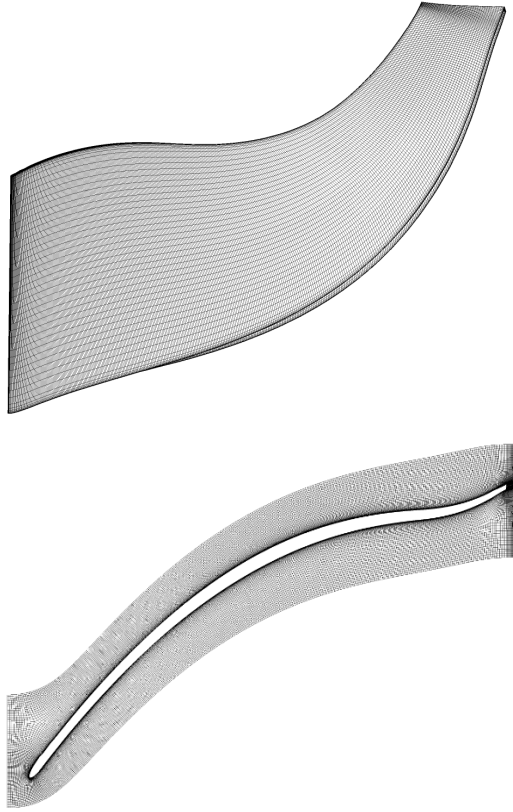
Figure 3. Computational mesh detail for Eckardt impeller A, upper: blade surface mesh; lower: blade to blade view mesh.
