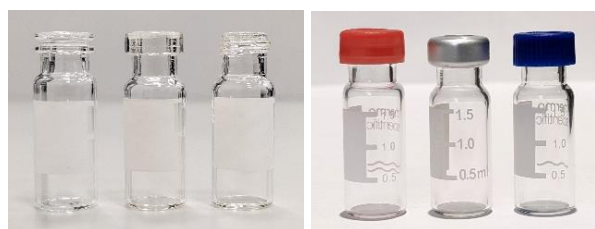
Fig. 1. Snap cap, crimp cap and screw cap vials. Left: Uncapped. Right: Capped.
