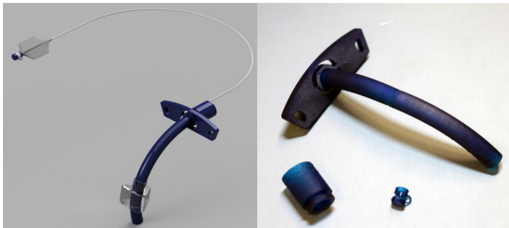
Figure 35. On the left-hand side a 3D computer aided design (CAD) from GrabCAD of a tracheostomy tube and on the right-hand side the subsequent print using the antimicrobial mix.
