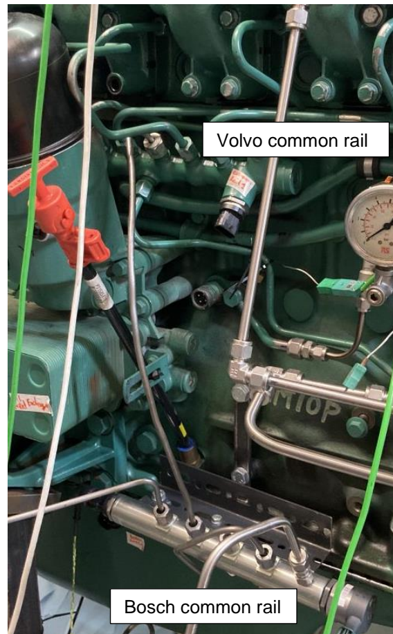
Figure 3.8: D8k commons rails and fuel supply pipework for the injectors
