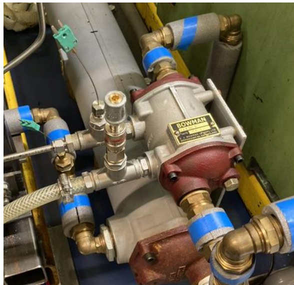
Figure 3.14: Small 4 kW heat exchanger for the fuel spill above the larger 72 kW exchanger for the engine coolant.
