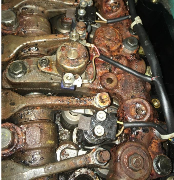
Figure 3.1: Overhead view of the D8k valve rockers and Jake brake control prior to reassembly, evident is the severe rust and corrosion.
