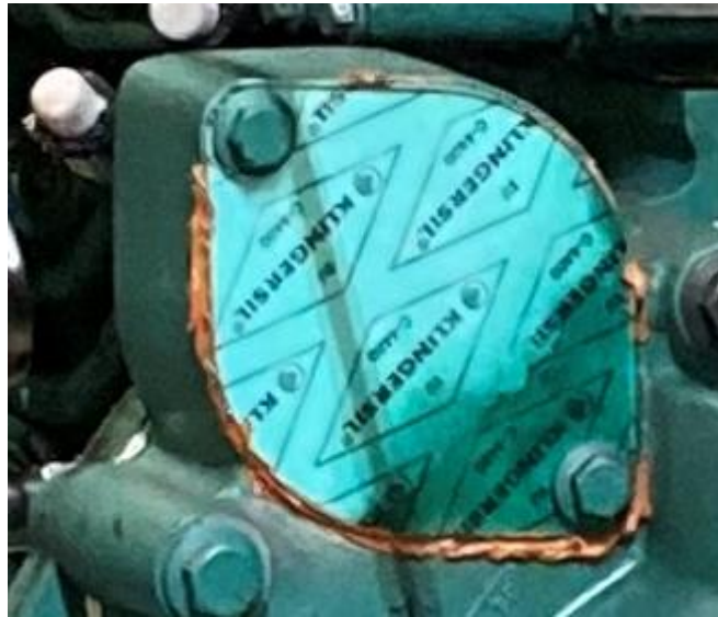
Figure 12.10: Steering manifold blanking plate with sealant to prevent oil leaks.
