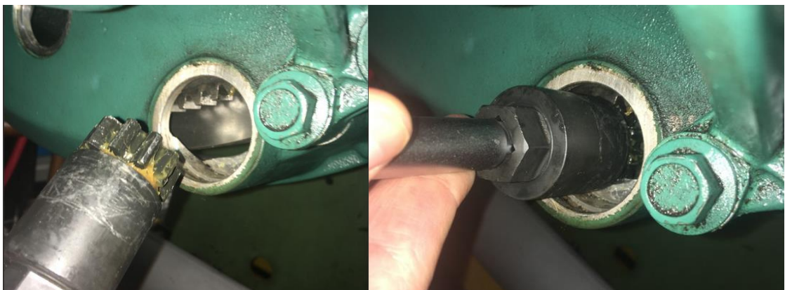
Figure 3.2: Cranking adapter for Volvo FE coach flywheels not centred with the intended flywheel access location.
