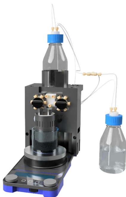
Fig. 5 Increased scale set-up, showing the arrangement of tubing to allow for increased volumes of reagents to pass through the system
