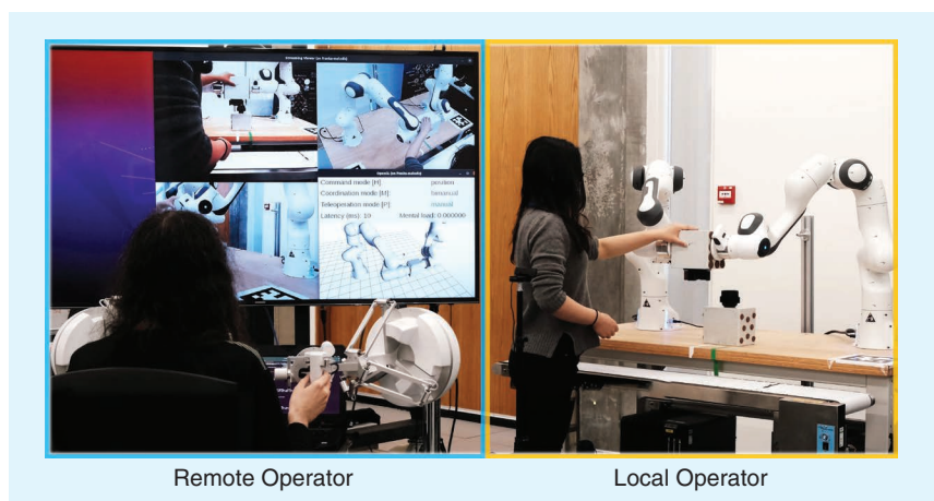
FIGURE 1. Real-world part assembly task performed via teleoperation and direct physical interaction using the proposed collaborative bimanual manipulation framework.
