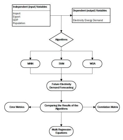
Figure 1. ML modelling framework proposed to estimate electricity demand.
