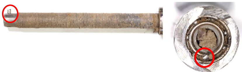
FIGURE 2. Detailed visual examination of internal components lead screw (left) and lower magnet cup (right) in a rod with a pin fracture. Circled in red: the pin.
