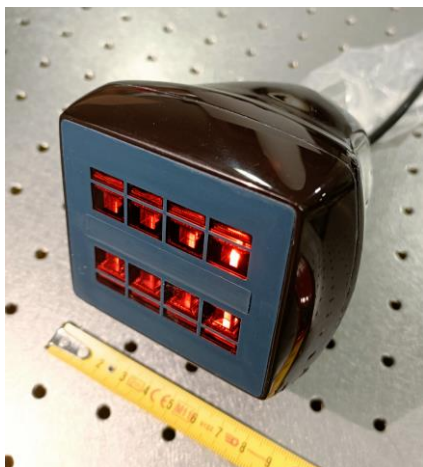
Figure 1 (Left). The SOLUS probe. Each red window corresponds to an optode, the central component is the US transducer.
