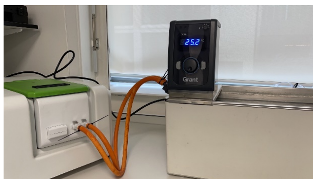
Figure 2.3 Setup for ground state absorption spectroscopy connected with a water bath for temperature dependence measurements.
