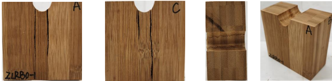
(a) Failure mode V
