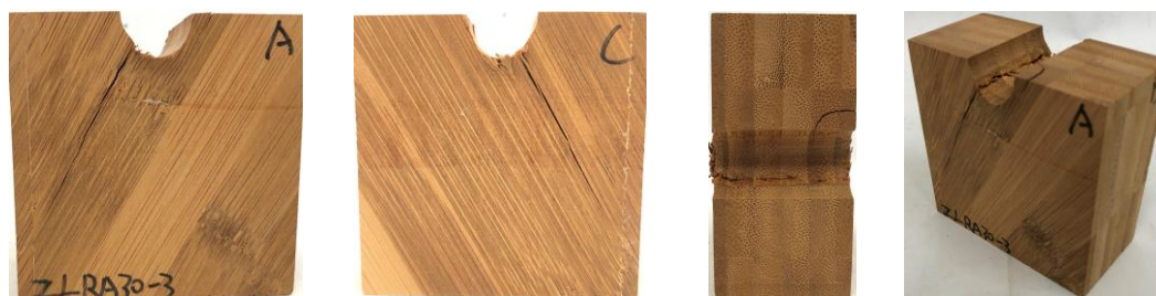
(b) Failure mode II
