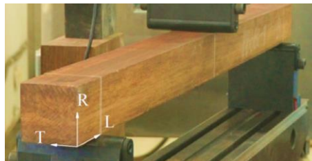
Fig.2 Bending test for PBSL (L is longitudinal direction; R radial direction, and T the tangential direction).
