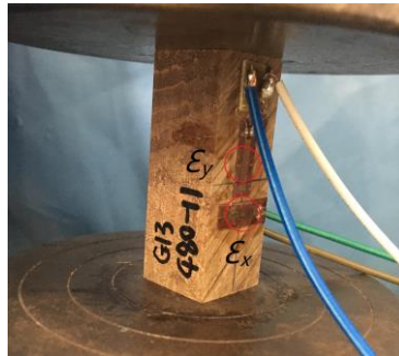
(b) Attachment method of Strain gauges
