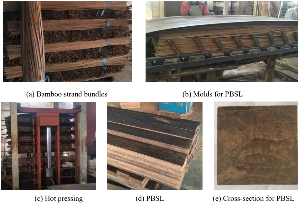
Fig. 1 Main manufacturing process for PBSL (Li et al. 2019c)
