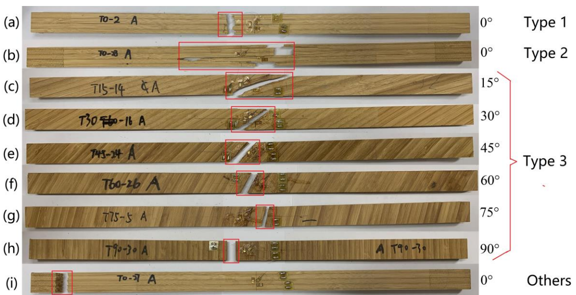
Fig.3 Typical failure types for specimens with different fiber alignment angles
