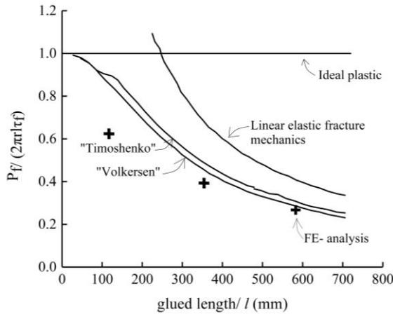
(a) Comparison of different methods (according to GIROD engineering model) [47]
