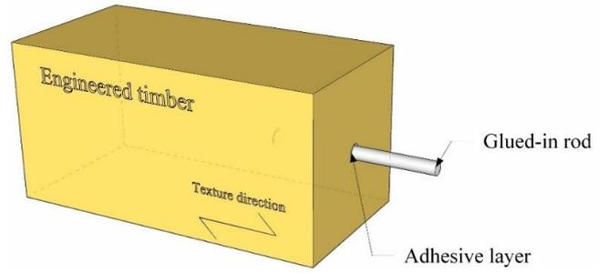
(c) Schematic diagram of single GIR connection
