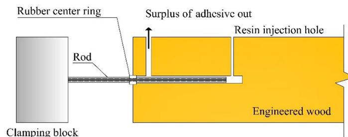
Fig.9 One of the available methods of gluing-in rods [99]
