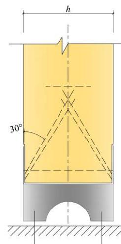
(b) Joint of the column with foundation [128]
