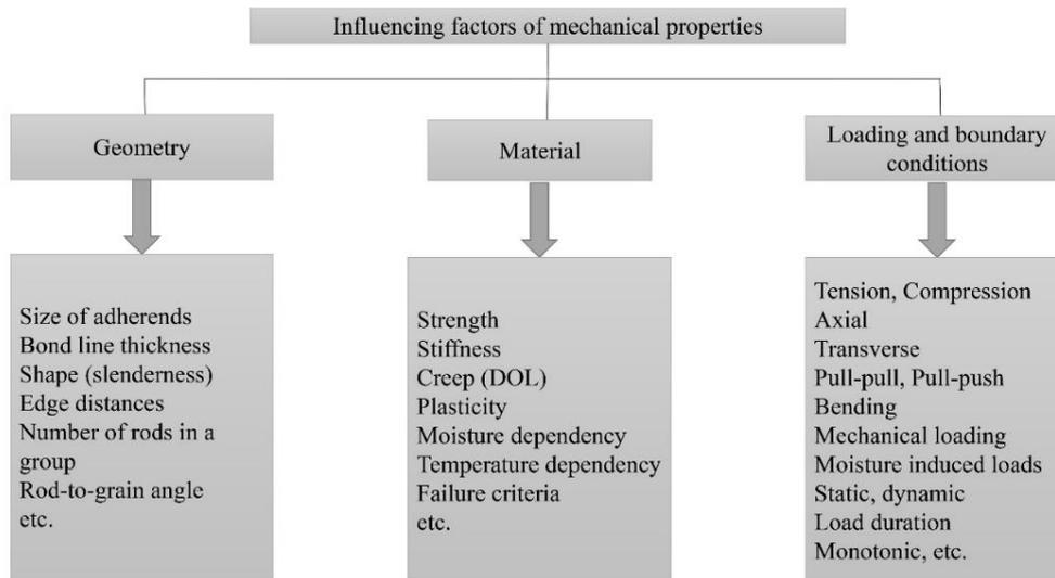
Fig.3 Influencing factors on the bond performance of glued-in connection [27]
