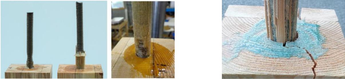
(a) Single rod yielding (left); shear block failure (middle); bond failure (right) [32]      (b) Splitting of timber (single rod connection) [36]
