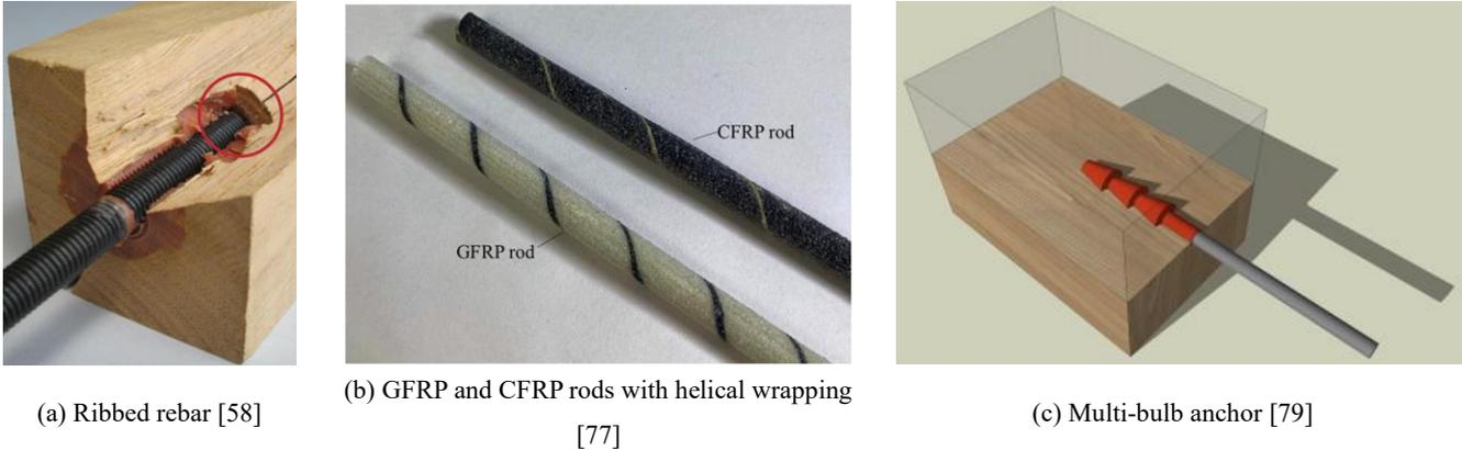
Fig. 7 Several illustrations of reinforcement in GIR connections
