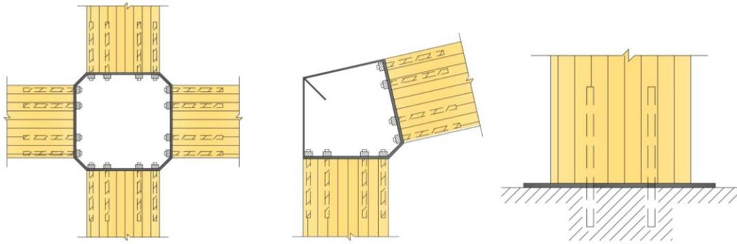
Fig. 11 Examples of applications of connections with glued-in rod [109, 119, 120]
