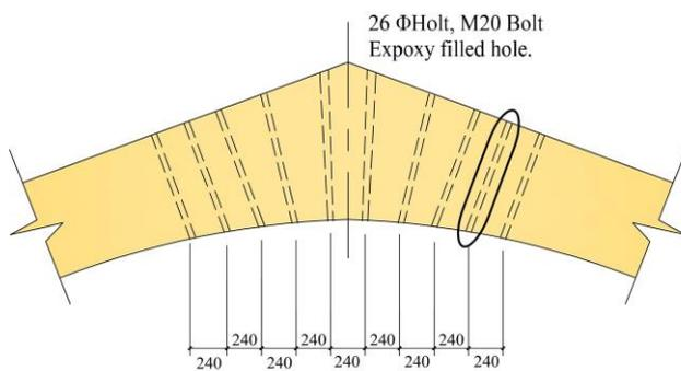
(e) Repair of a curved glulam beam with epoxied steel dowels [130]
