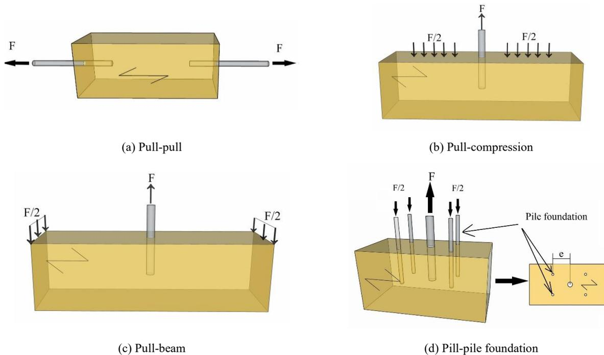
Fig.8 Several loading and boundary conditions
