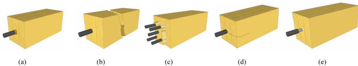
Fig.14 Types of failure modes of glued-in rod connections
