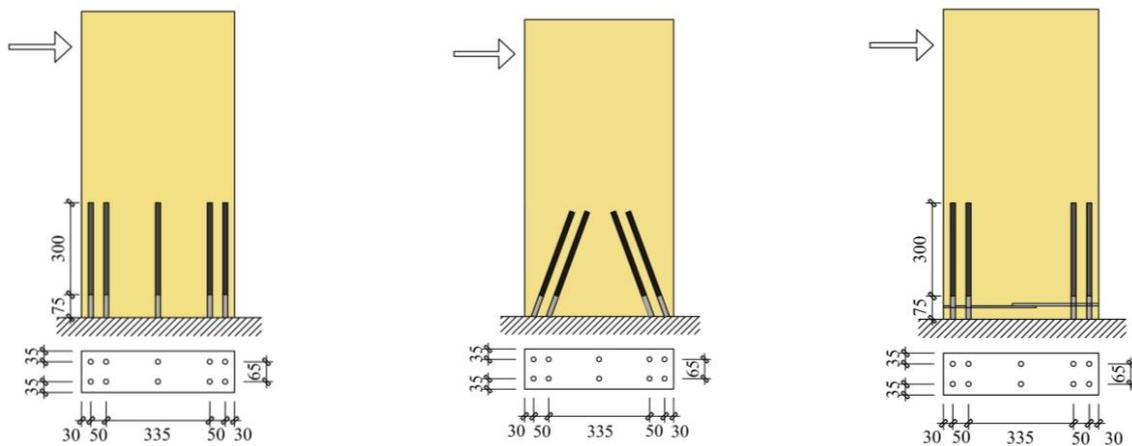
(a) Multiple GIR in the grain direction [25]    (b) Multiple GIR at an angle of 20° [25]    (c) Multiple GIR with stirrups [25]
