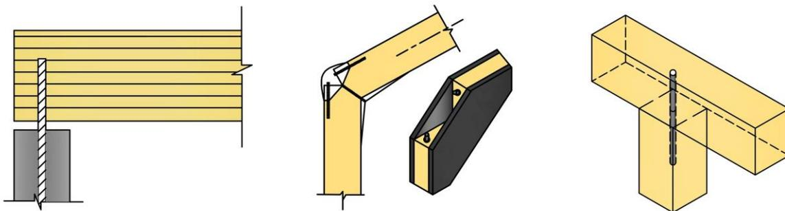
Fig.12 Examples illustrating some of the possible connection methods employing bonded-in rods
