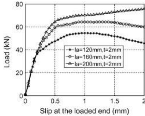
(b) Curves of load-deformation with different anchorage lengths [44]
