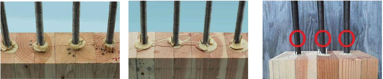
(c) Multiple rod bond failure [118]      (d) Multiple rod splitting [118]      (e) Multiple rod yielding [118]
