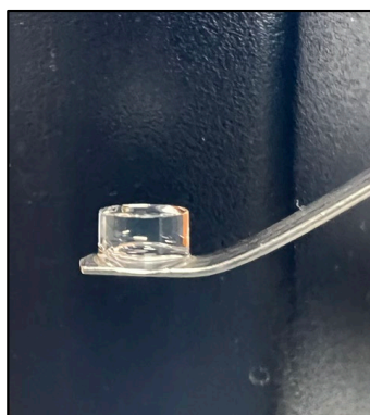
Figure 1. A picture of a photo-crosslinked GelMA hydrogel sample after it was removed from the 96-well plate.
