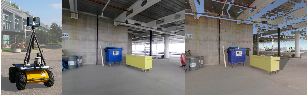
Figure 1: Left: Husky robot platform with mounted FARO Focus M70 scanner. Middle: Rendering from Ricoh Theta Z1 360° camera in the Unity interface. Right: Rendering of FARO pointcloud in the Unity interface. In the proposed framework, photorealistic is captured and localised autonomously and can readily be reconstructed in the Unity interface.
