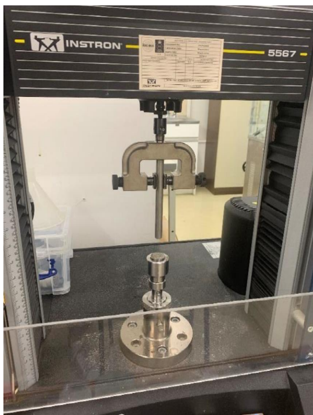
Figure 5-2 MN array mechanical testing setup using an Instron tensile tester. A cylindrical probe attached to the upper instrument frame.
