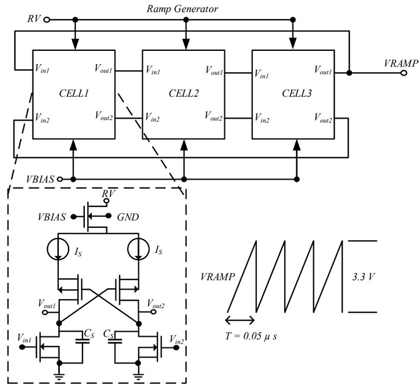
Figure 8. Accurate ramp generator circuit for VRAMP.
