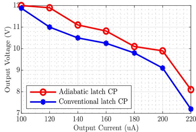
**Figure 14.** Comparison of the output voltage of the conventional and adiabatic charge pumps for 100 to 220  $\mu\text{A}$  output current. In each, the total capacitance used is 60 pF.
