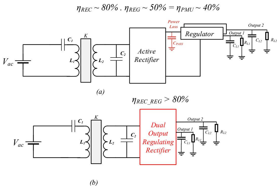
**Figure 1.** Block diagram of (a) conventional WPT system with  $C_{PASS}$  between two stages of regulation and rectification (b) single stage dual output regulating rectifier.
