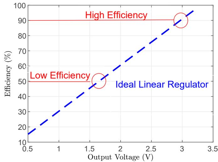
Figure 2. The LDO efficiency ( $V_{out}/V_{in}$ ) of regulator changes over various output voltage.
