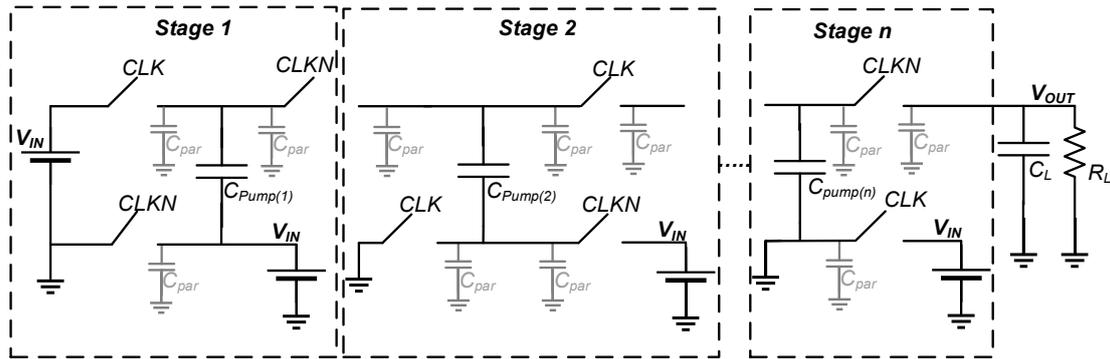
Figure 10. Linear charge pump with  $n$  stages.
