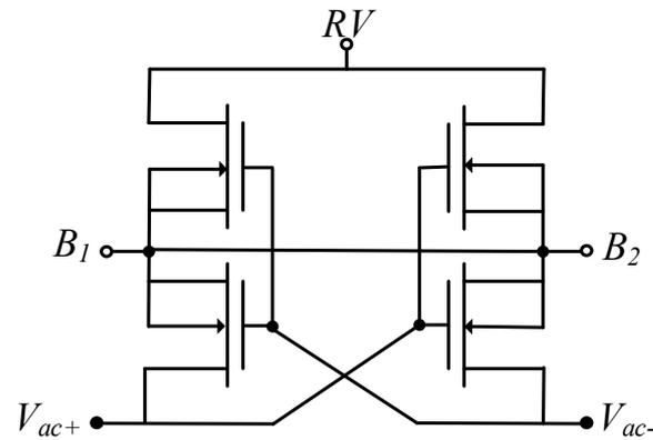
**Figure 6.** Adaptive body biasing (ABB) with  $B_1$  and  $B_2$  connected to the body of  $pMOS1$  and  $pMOS2$ , respectively.
