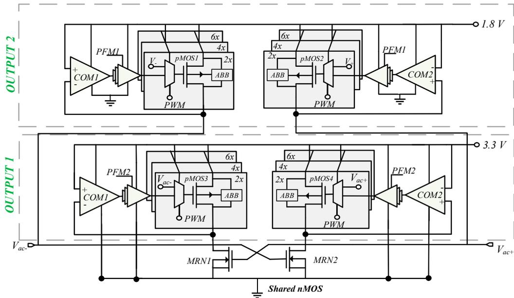
Figure 4. Proposed dual output regulating rectifier with PWM/PFM event-driven feedback control.
