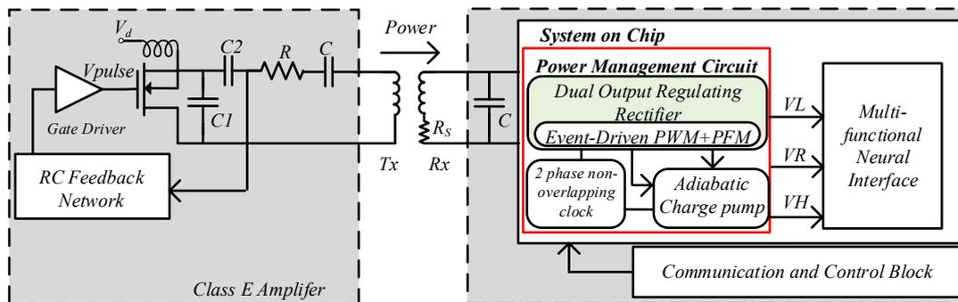
Figure 3. Proposed WPT system for a neural interface implantable device.
