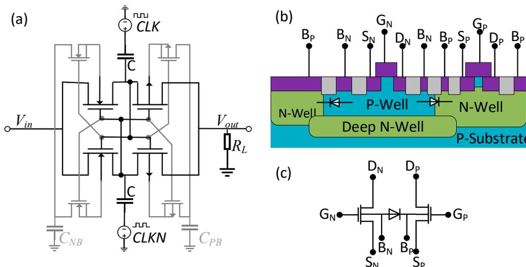
Figure 12. (a) Dynamic bulk biasing (in grey) with the charge pump design (b) physical implementation to the latch-up (c) parasitic diode between the bulk of pMOS and nMOS transistors.
