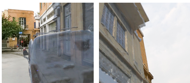
(A) A car captured in the mesh model which was no longer on-site at the time of our test. (B) An extreme case of poor tracking causing misalignment between the model and the real building
