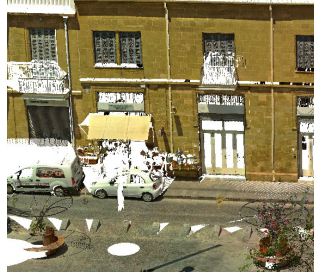
Figure 5: Dense laser point cloud model from a FARO scanner.
