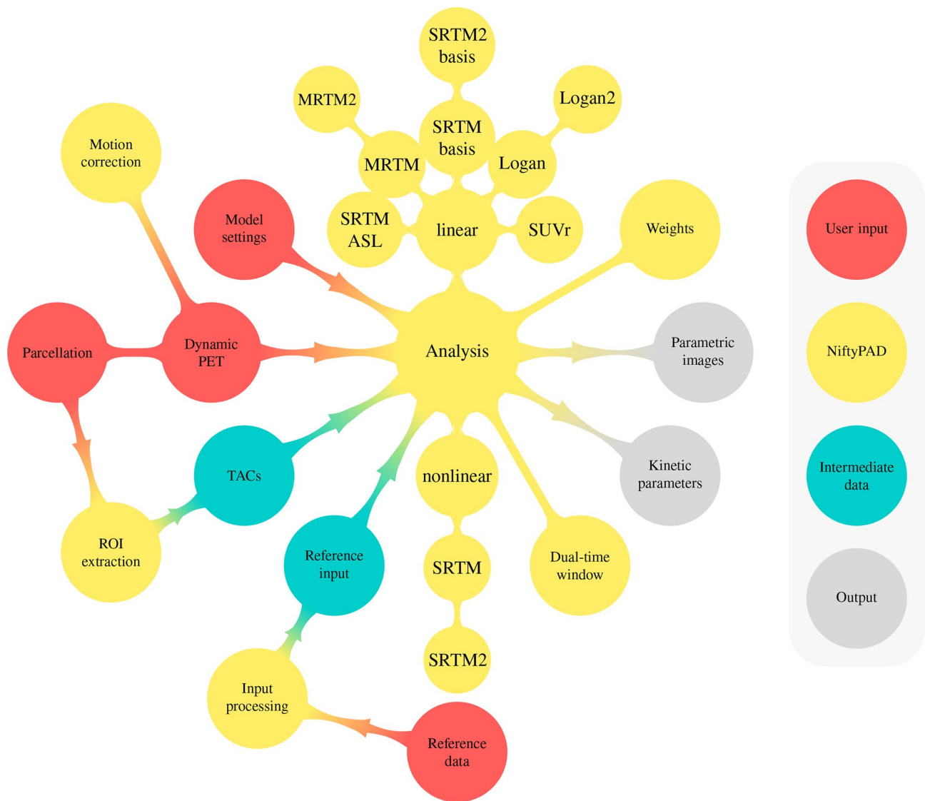
Fig. 1 Features of NiftyPAD and its workflow. The features and functions NiftyPAD provides are shaded in ●, including optional motion correction, reference input processing, a group of kinetic modelling
