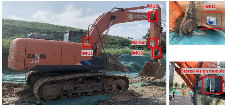
841 Fig. 13 Large excavator and the installation of the onboard devices
