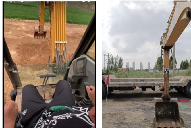
397 (a) The actual operator's view. (b) The view of the stereo module.
