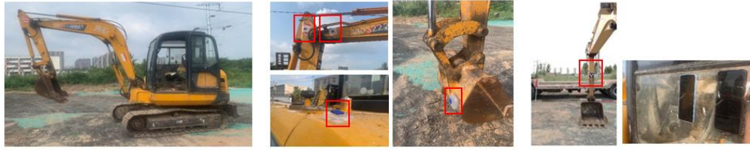
(a) The excavator (b) The IMUs installed on the excavator (c) The stereo module and the fiducial marker
