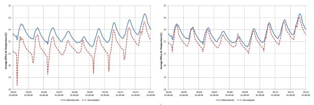
Figure 3 Monitored & simulated office temperature in 2<sup>nd</sup> period: initial model (left), 1<sup>st</sup> calibrated model (right)
