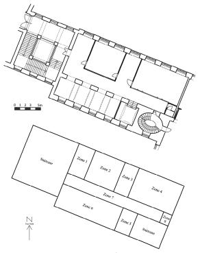
Figure 1 Building floor plan and thermal zoning of the model
