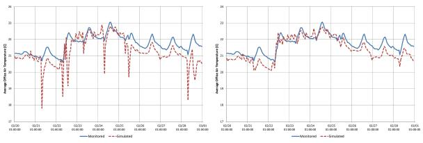
Figure 2 Monitored & simulated office temperature in 1<sup>st</sup> period: initial model (left), 1<sup>st</sup> calibrated model (right)
